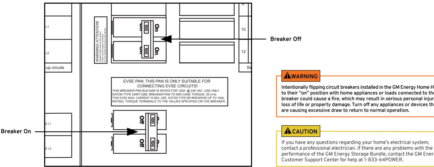
Intentionally flipping circuit breakers installed in the GM Energy Home Hub to their "on" position with home appliances or loads connected to the breaker could cause a fire, which may result in serious personal injury, loss of life or property damage. Turn off any appliances or devices that
