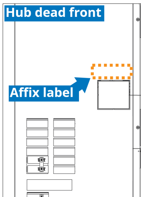
Figure 124: Location to apply MAIN SERVICE DISCONNECT label
