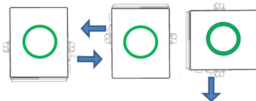
Definition: To ensure that the product will not be splashed by water, the direction of the wire outlet is not restricted when wall-mounted installation.
