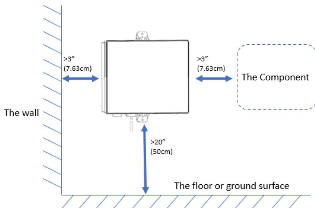
Installed on the ground > 50cm (20" inch), the distance between the wall and other components is > 7.63cm (3" inch)
